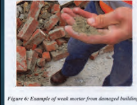
Figure 6: Example of weak mortar from damaged building.
