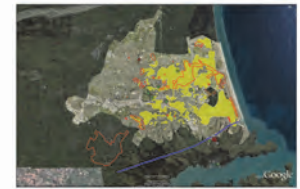
Figure 2. Liquefaction in February 2011 (green) and September 2010 (red contours) (courtesy of R. Green, (EERI 2011))
