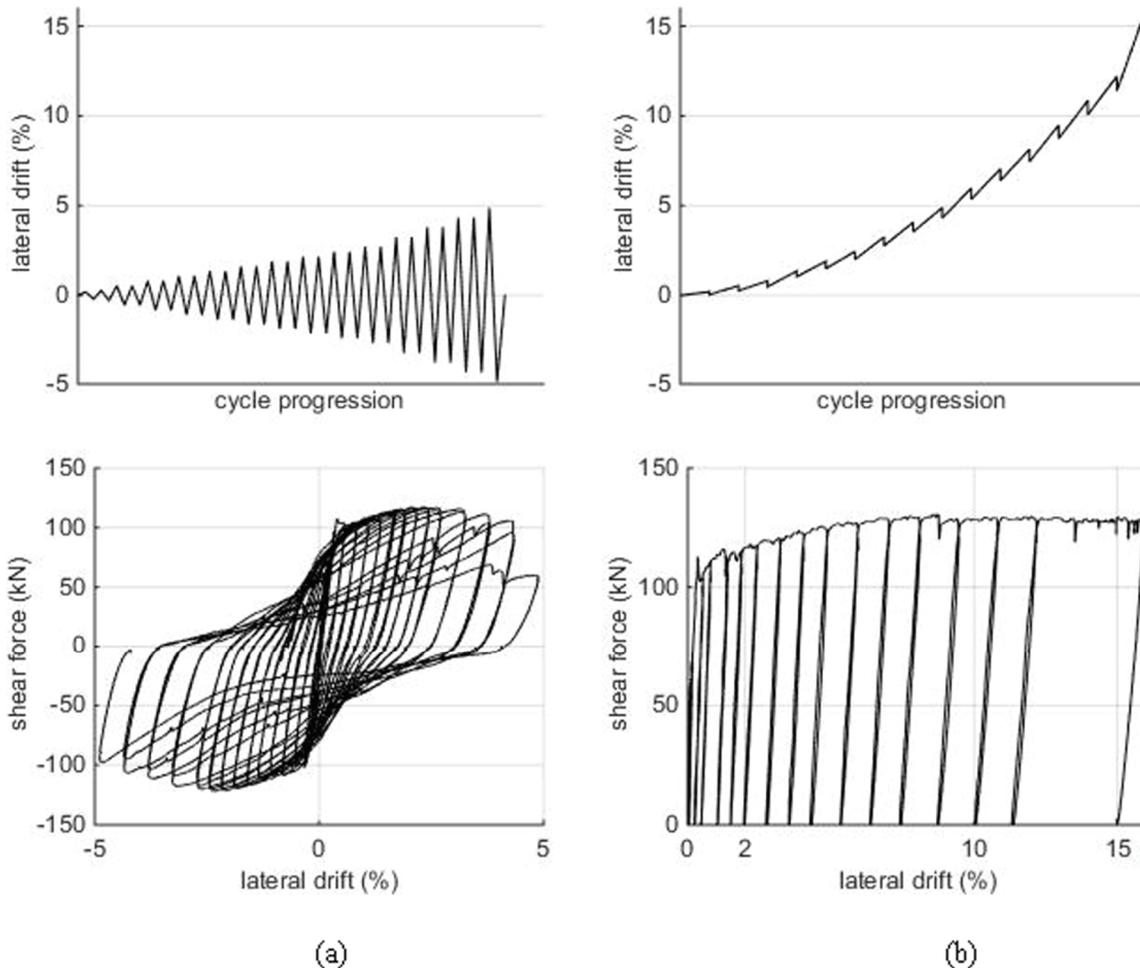
Figure 4. Loading protocol and shear force vs lateral drift for specimen Cyc (a) and Mono (b).
