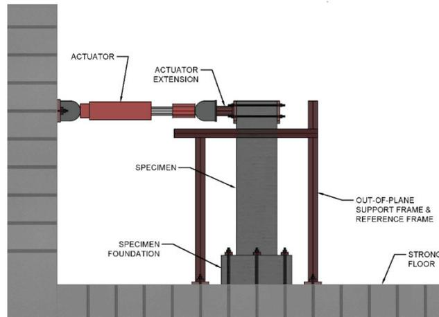
Figure 2. Rendering of test set-up
