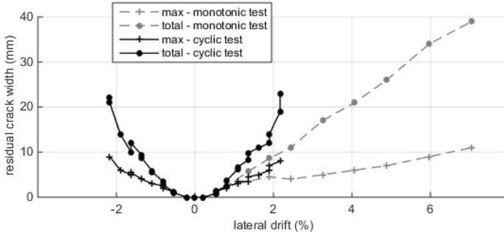
Figure 5. Residual crack widths (maximum and total) for specimen Cyc (black) and Mono (grey).
