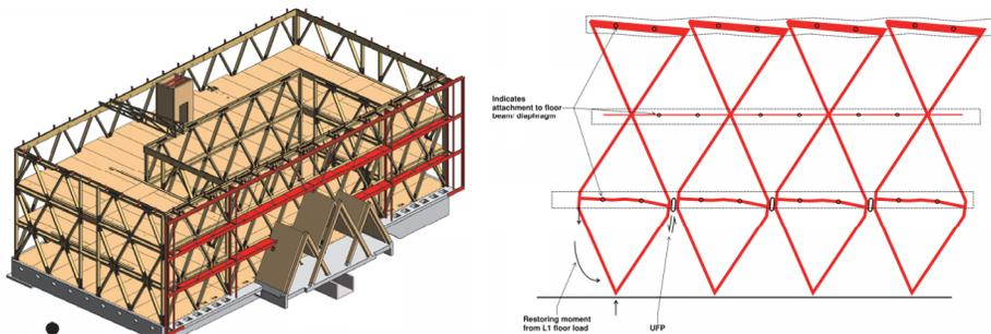
Figure 9. Render of structure and illustration of actions on ductile diagrid.
