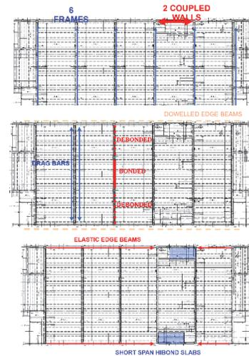
Figure 3. Exterior view. ,Plan on seismic systems, diaphragm actions transversely, and longitudinally
