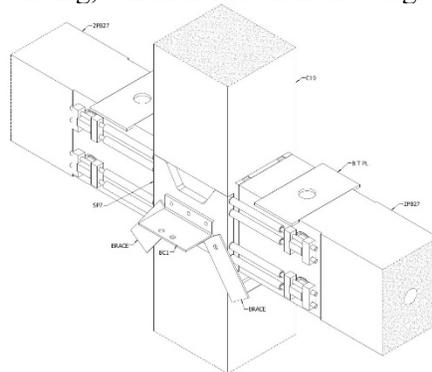
*Figure 10. Isometric of beam/column joint from Alan MacDiarmid.*
