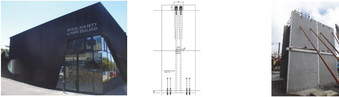
Figure 5. External view and typical rocking wall arrangement, and walls during construction.
