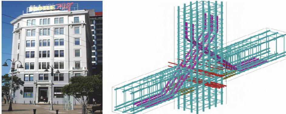
Figure 7. Exterior view of Huddart Parker, and slotted beam reinforcement arrangement.
