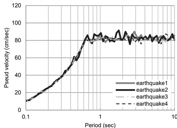
Figure 11. Pseud velocity spectrum of input ground motion.
