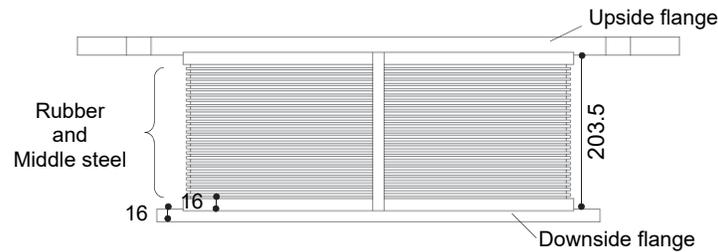
Figure 4. Specimen for rotary deformation test.
