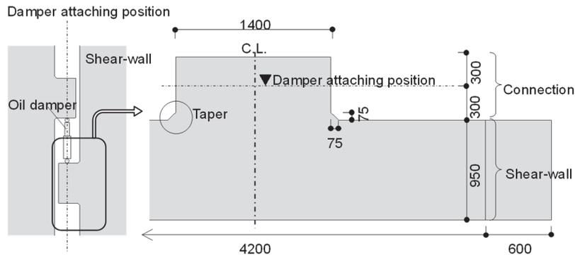
Figure 8. Specimen for cyclic loading test.
