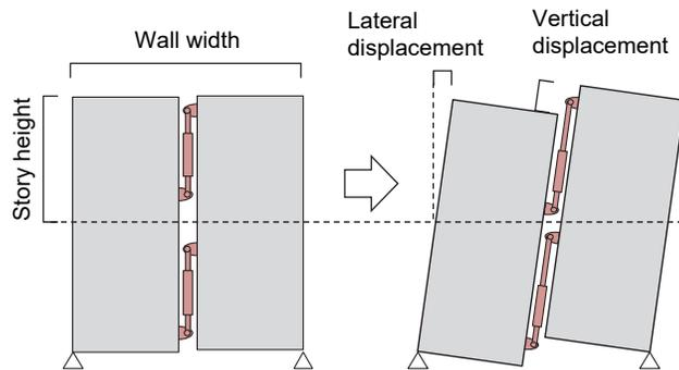
Figure 3. Conceptual diagram of amplification of oil-dampers deformation.
