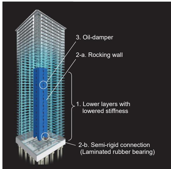
Figure 1. Perspective drawing of the system.
