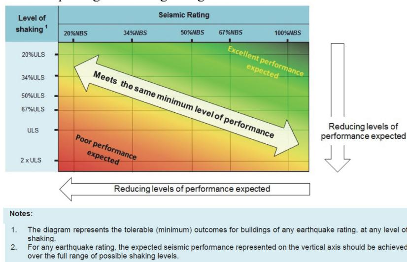
Figure 2. Diagram used to convey uncertainty in the New Zealand Seismic Assessment Guidelines
