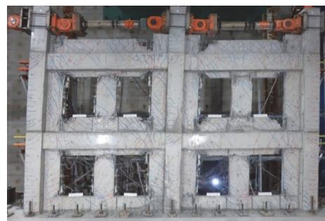
Photo 2. Damage state at  $R=3.0\%$
