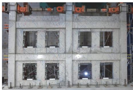
Photo 1. Damage state at  $R=1.0\%$
