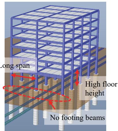
Figure 4 Structural characteristic of over-track buildings
