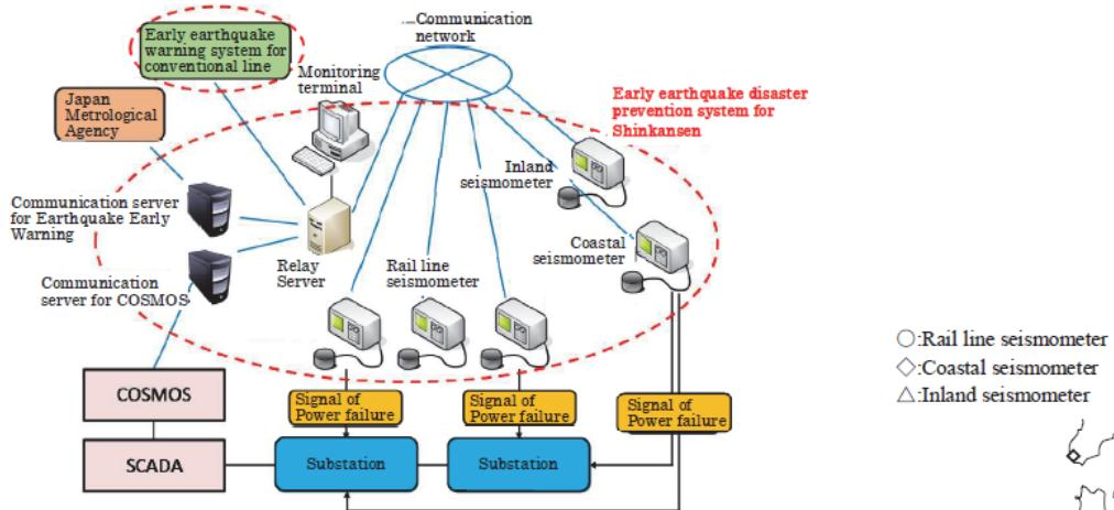
Figure 1 Earthquake detection system
