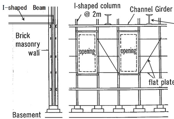
Figure 10 Typical Steel Structure Frame
