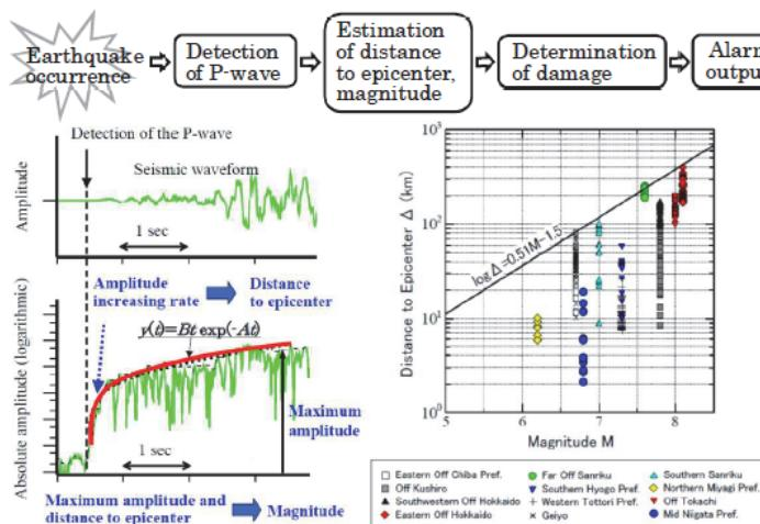
Figure 2 Processing flow of Primary wave alarm<sup>1)</sup>
