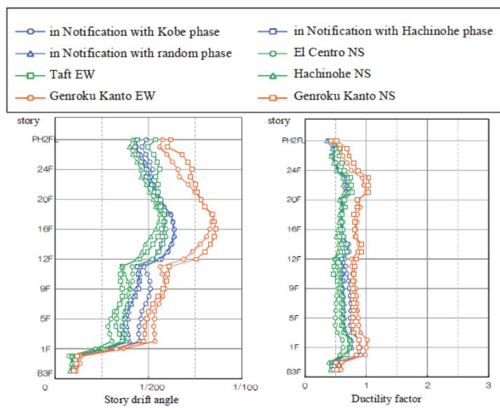
Figure 7 Seismic response (Level 2 earthquake)
