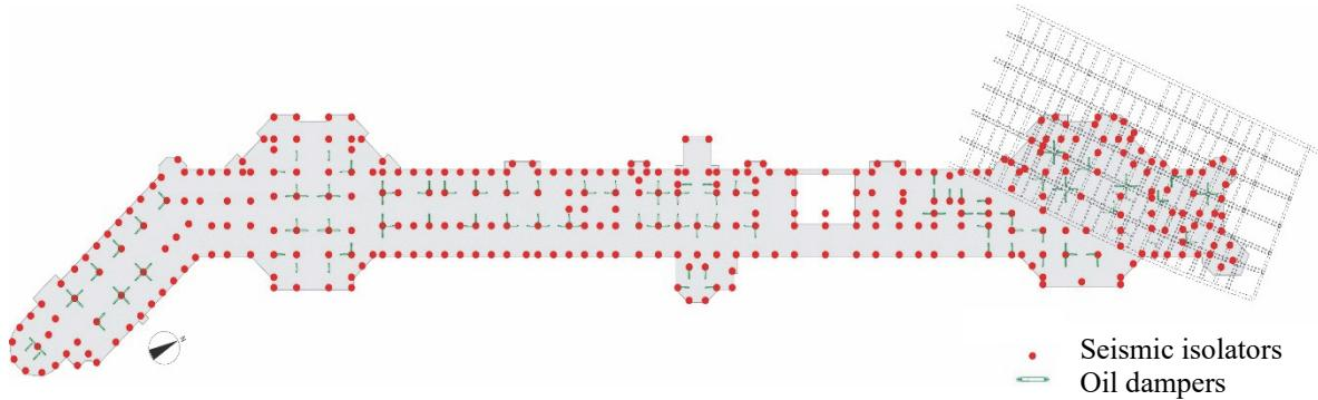
Figure 12 Layout of seismic isolation system
