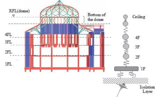
Figure 14 Lumped mass system model
