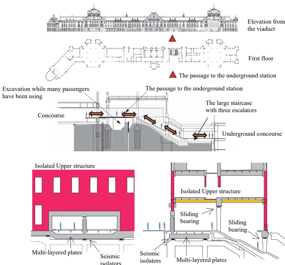
Figure 16 Solution of seismic isolation system for passenger traffic
