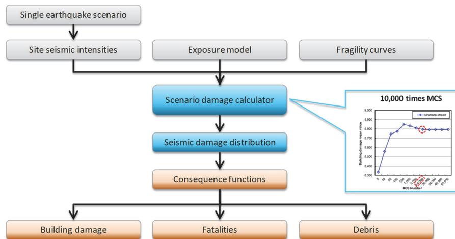
*Figure 2. The process and outputs at each state of the probabilistic risk analysis.*
