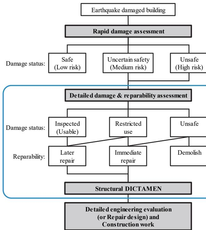
Figure 7. Seismic damage assessment flow.
