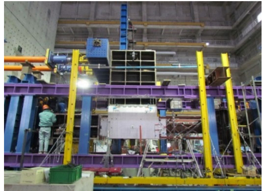
Full-scale experiment on a pile with pile-cap
