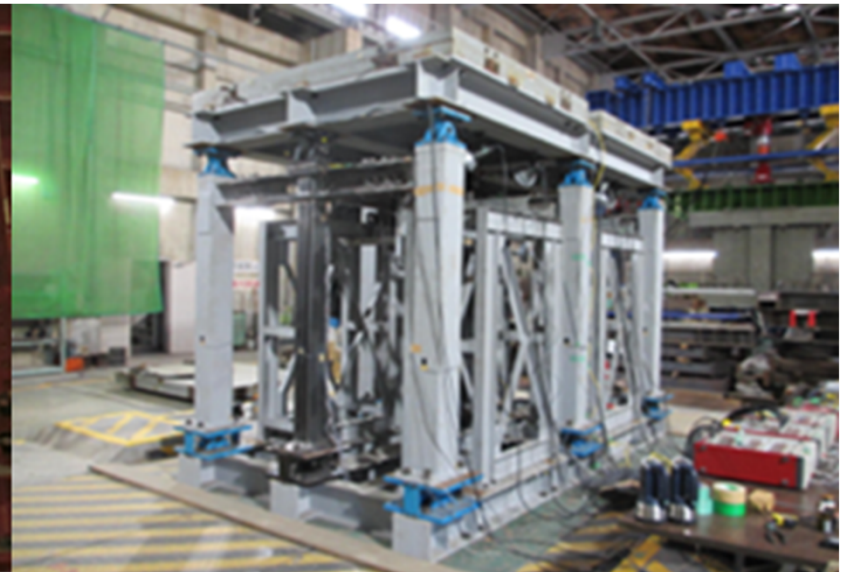
Photo 4. Shaking table test on two-bay frame
