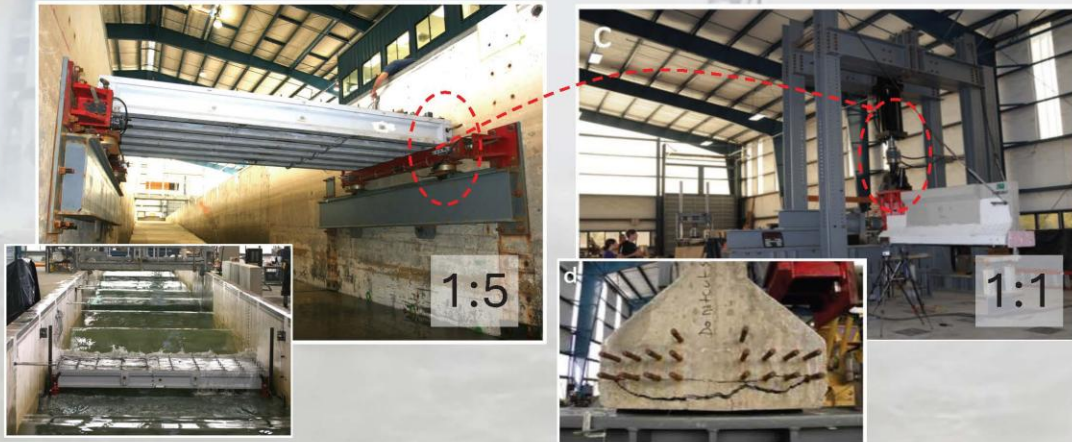
Hydraulic model study of a 1:5 scale bridge deck section subject to storm surge and waves.
