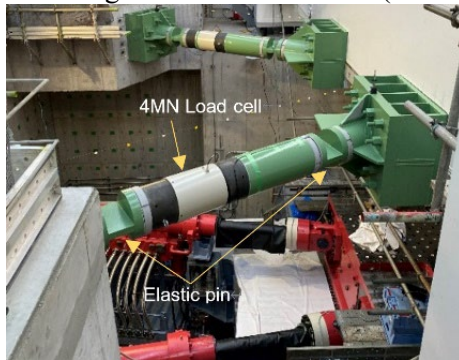
(a) V-shaped measurement links
