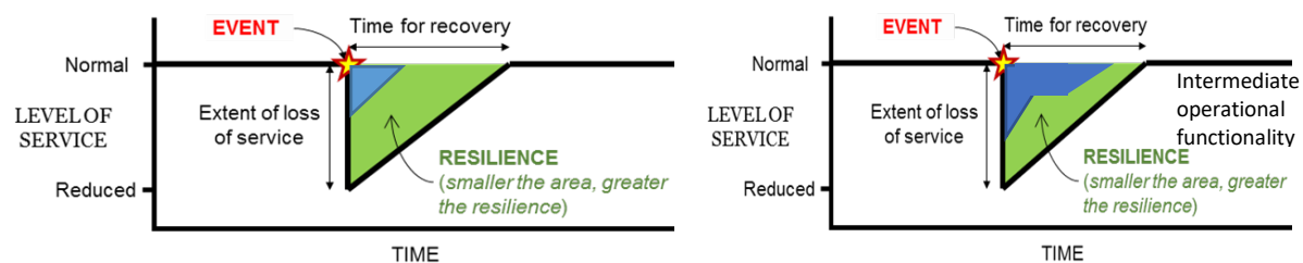
Figure 4. (a) Left: Enhancing Resilience through reduced reduction in functionality and rapid return to service (as indicated by blue triangle) (b) Right: Staged recovery of functionality over time
