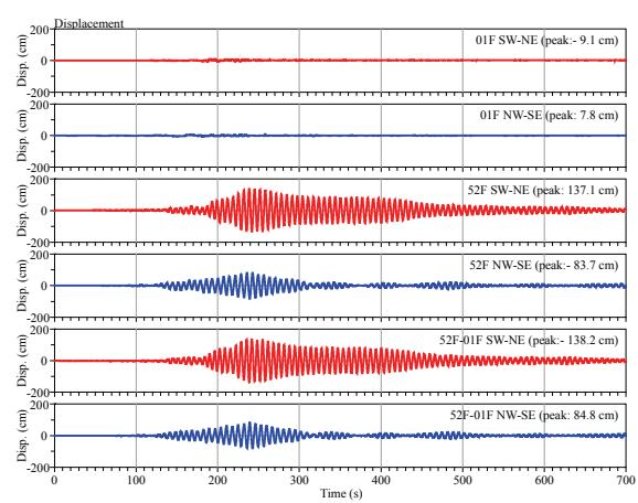
Figure 2. Recorded strong motion of 52+3 storied steel office building located 770km from the epicenter
