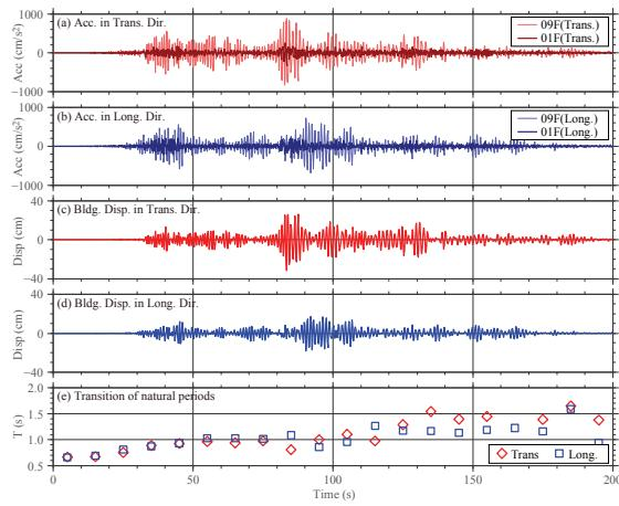
Figure 1. Recorded strong motion and the calculated fundamental natural period
