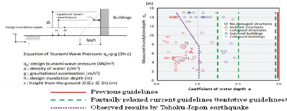
Figure 19. Estimated coefficient of water depth of detailed studied buildings
