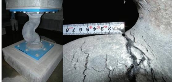
Figure 8. Lead damper cracked
