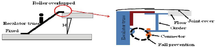
Figure 18. Prevention of fallen down of escalator truss
