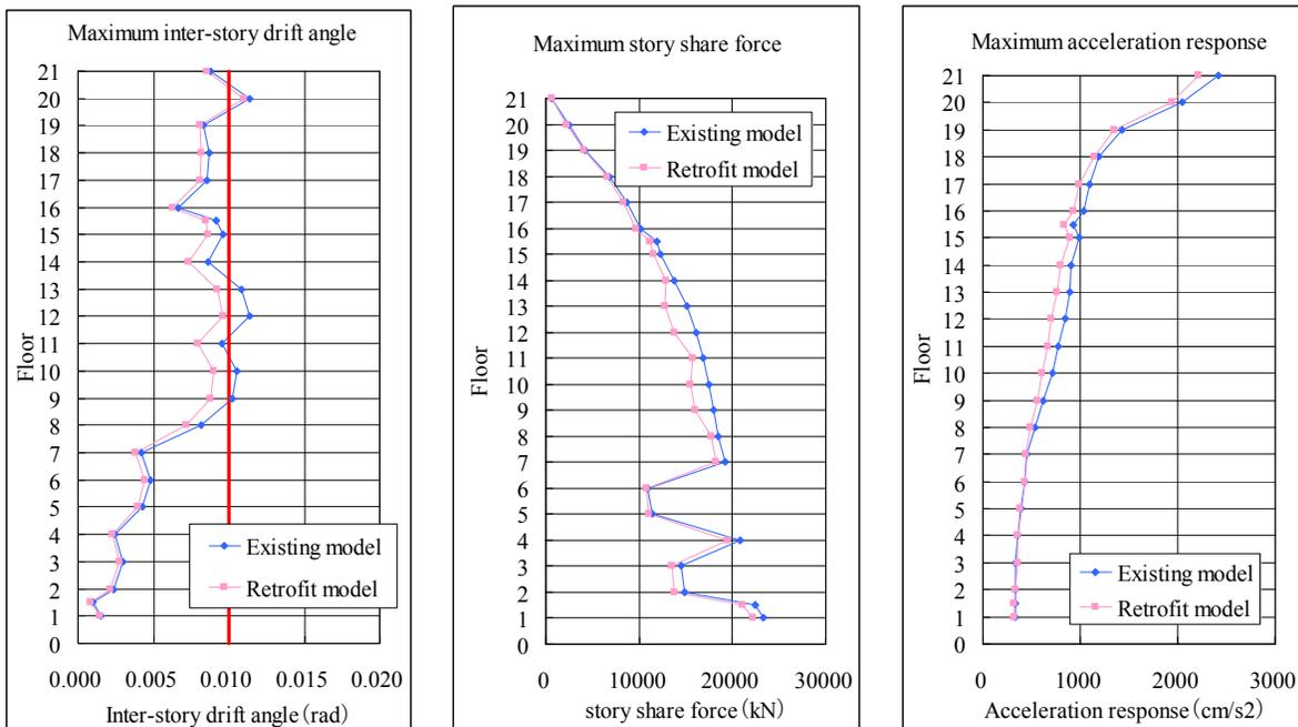
Figure 17. Maximum Response of Y-direction
