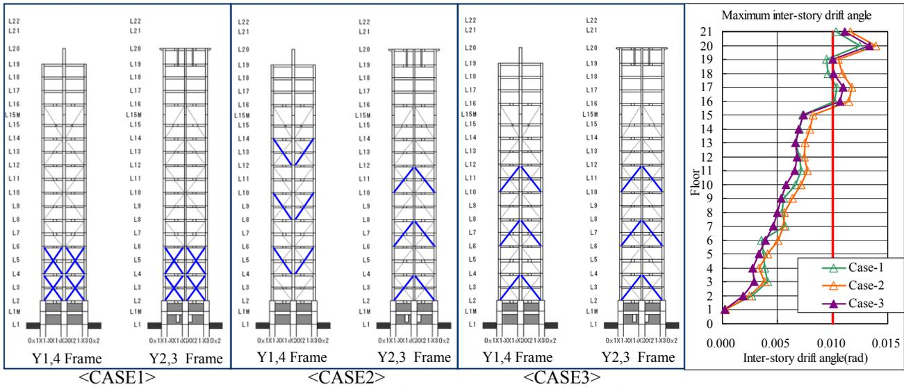
Figure 14. Damper disposition proposal of X-direction
