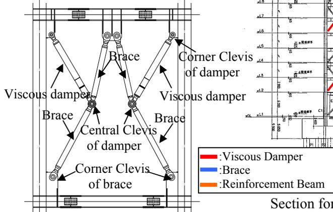
Figure 4. Amplification mechanism type
