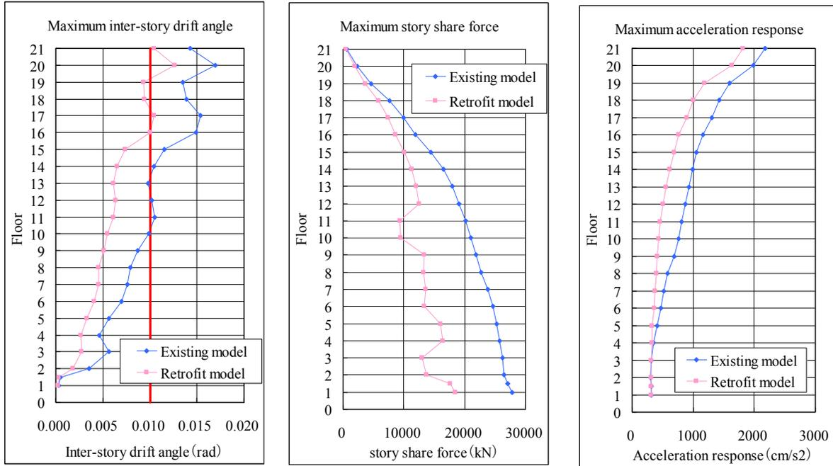
Figure 16. Maximum Response of X-direction
