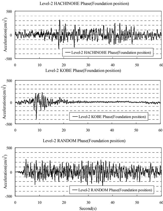
Figure 6. Acceleration history (Level-2, GL-5.5m)
