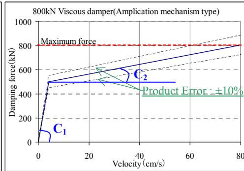
Figure 12. Nonlinear curve (Type-2 viscous damper)
