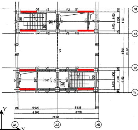
Figure 3. Beam plan for standard floor
