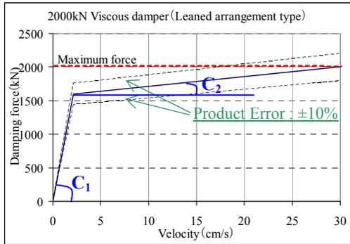
Figure 11. Nonlinear curve (Type-1 viscous damper)
