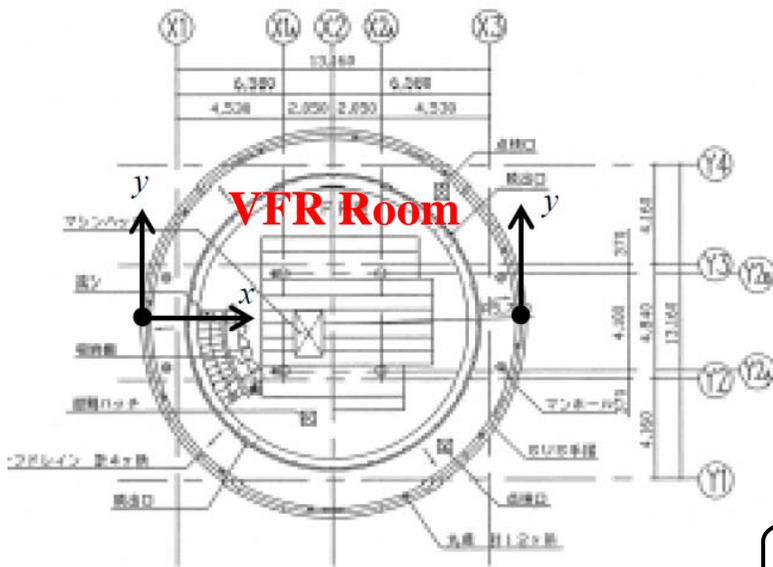
Fig. Seismographs arrangement
