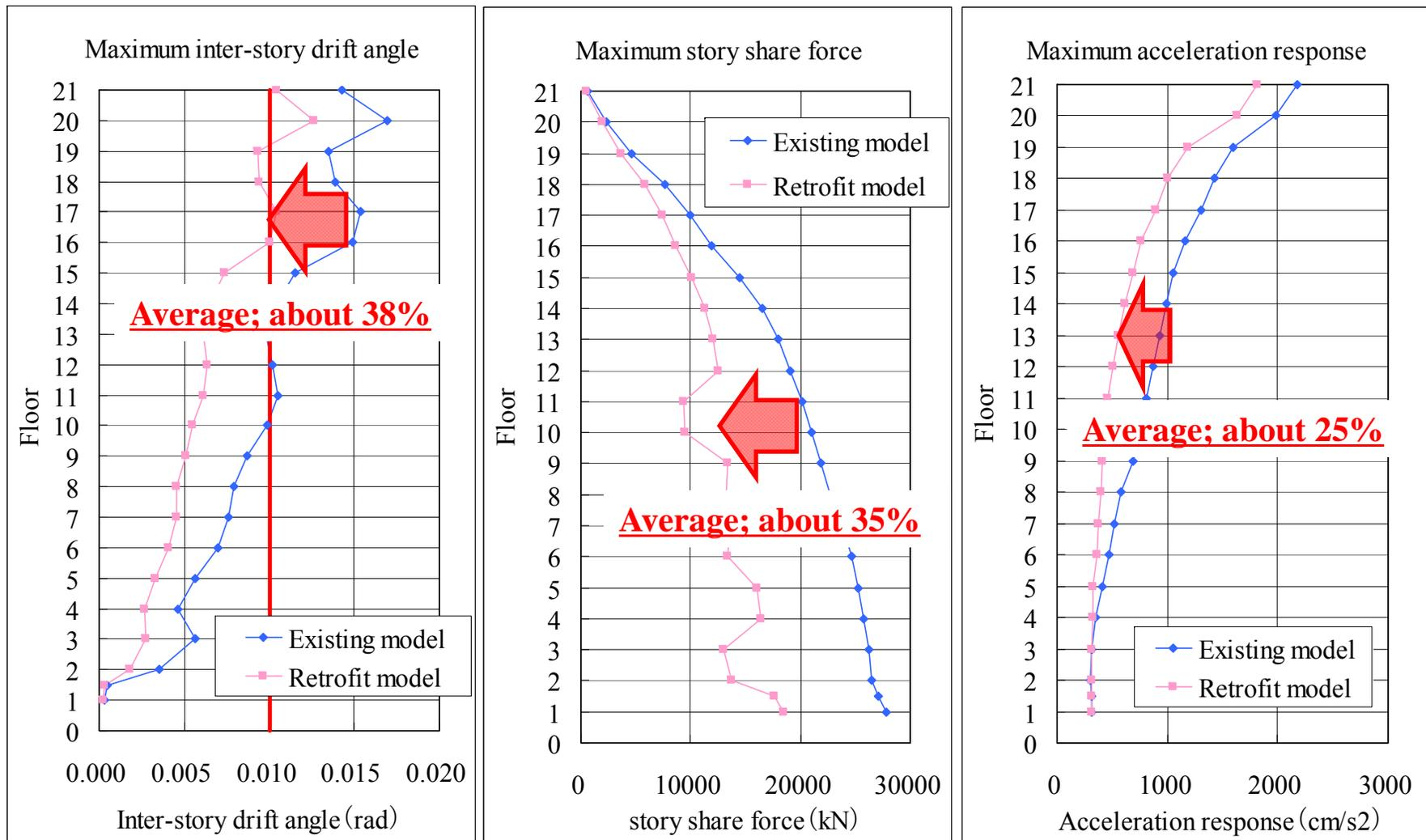
Fig. Maximum Response of X-direction
