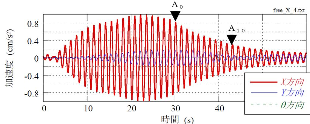
Fig. Free vibration of horizontal motion
