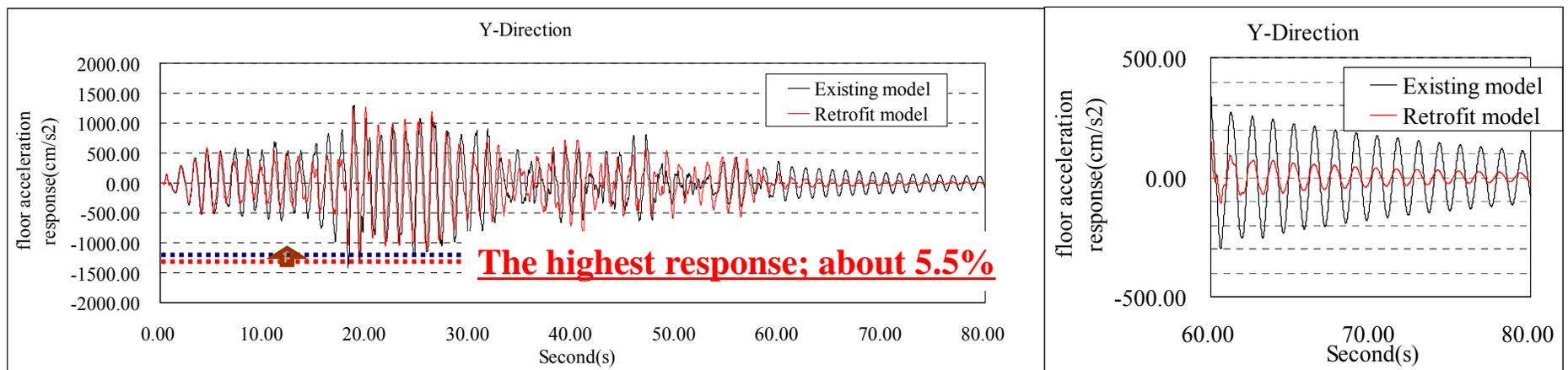
*Fig. Time History of Response acceleration (Y-direction / L20)*
