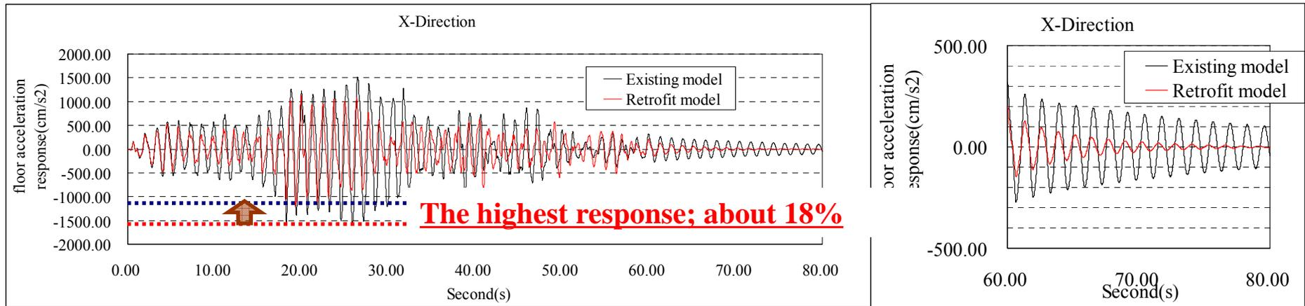
*Fig. Time History of Response acceleration (X-direction / L20)*
