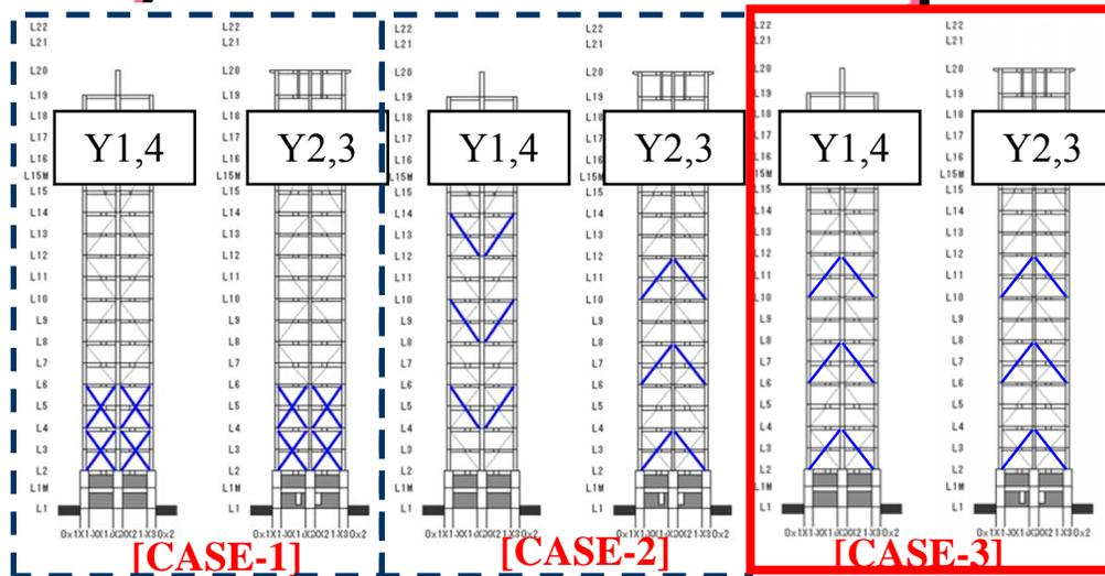
Fig. Damper disposition proposal of X-direction
