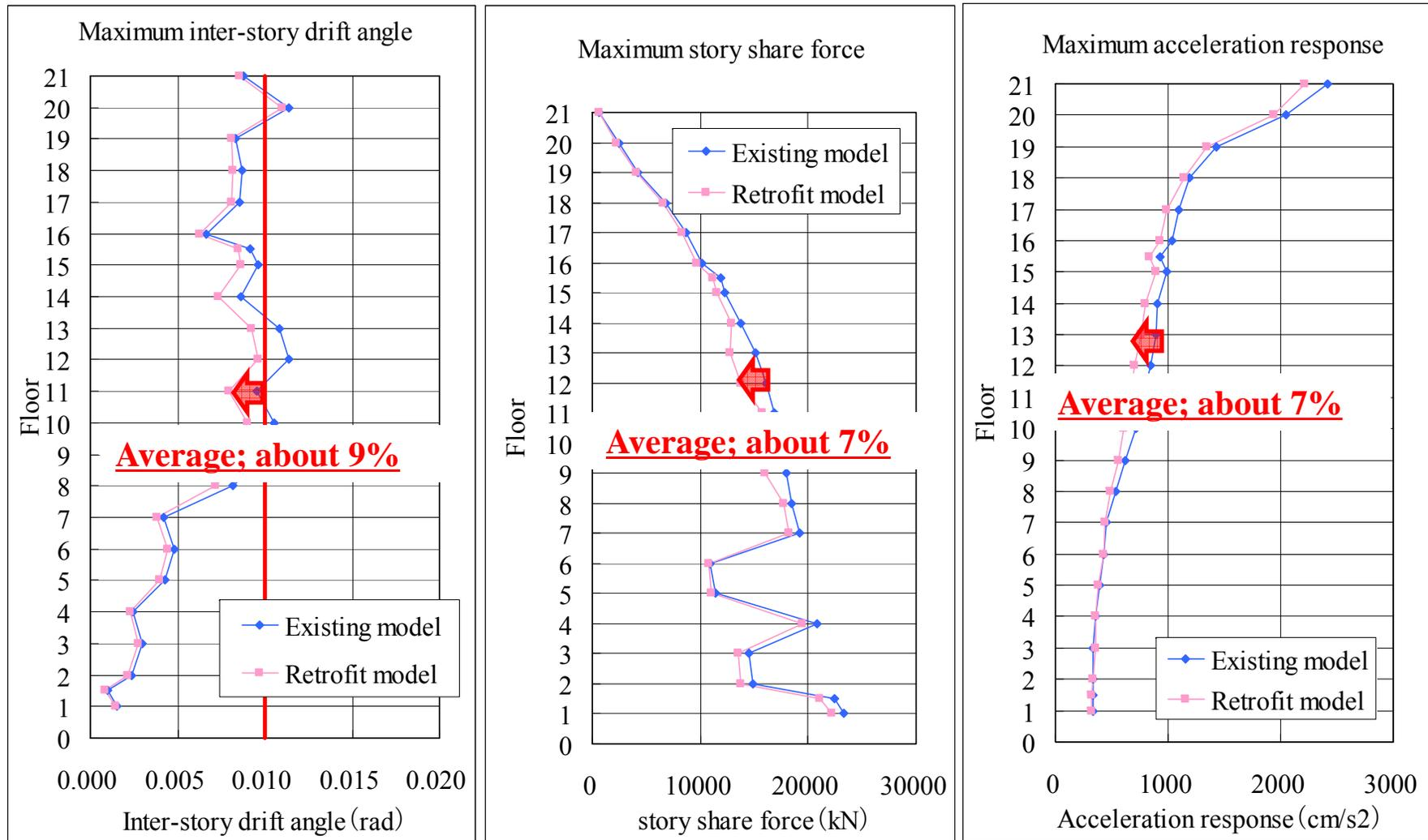
*Fig. Maximum Response of Y-direction*
