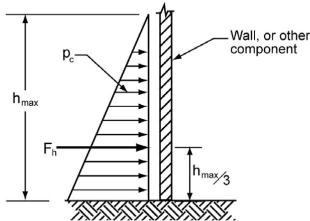
Figure 6-4 Hydrostatic force distribution and location of resultant.
