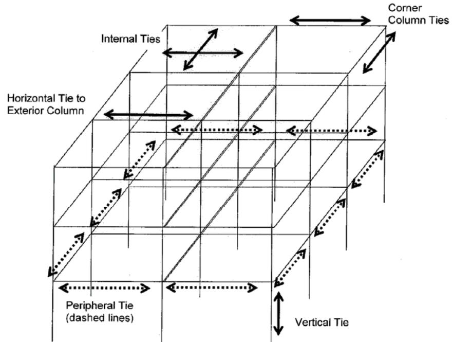
Note: The required Exterior Column, Exterior Wall, and Corner Column Tie forces may be provided partly or wholly by the same reinforcement that is used to meet the Peripheral Tie requirement.
