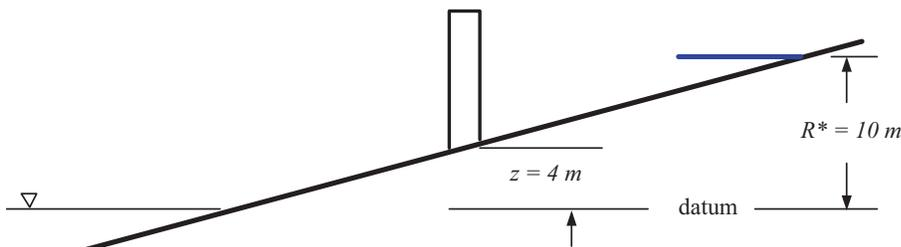
Figure C-1 Definition sketch for example calculations:  $R^*$  is the maximum runup elevation (the maximum inundation distance is 500 m) and  $z$  is the elevation at the location of the tsunami evacuation structure (located 200 m from the shoreline). Two horizontal lines represent the initial water level and the maximum inundation level, respectively.
