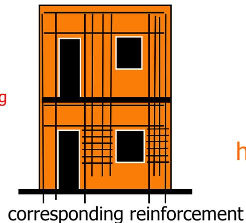
reinforce for sufficient inelastic deformation capacity in hinging regions
