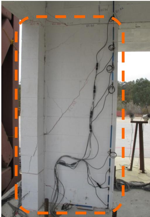
**Wall W - 3** was shear - dominated one way , flexure - dominated the other way , exceeded **1%** drift ratio
