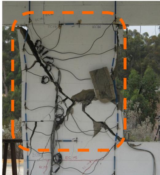
**Wall W - 2** was shear - dominated , exceeded **2%** drift ratio
